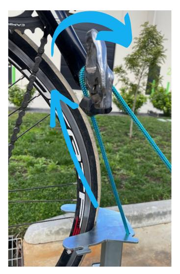
Loop rope fastening to the back of the extension and up over into the locking loop. 4) Press the seat of your bike into the rear bar to create a small amount of tension. This locks the bike into place
