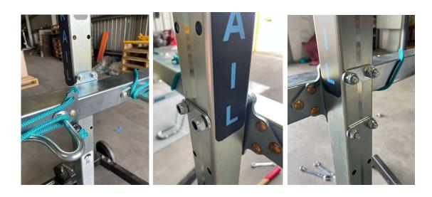
Step 6 – Install Top Tube using M10 bolts (#7). The "Single Trail" Sticker indicates correct orientation.
