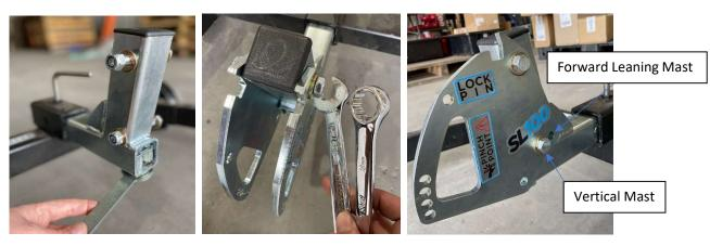
Step 2 – Install Upright Mast as shown by removing the M12 x 105mm (SL150) or M12 x 90mm (SL100) bolts and sliding it between the side plates. Rest the lock in position and re-install the M12 bolt through the plates and the bush attached to the upright (you may need a hammer to tap the bolt through). The M12 bolt needs to be moderately tightened, washers and bolts should NOT spin freely, overtightening can prevent pivot action.
