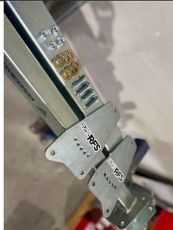
Install each side plate with the M12x30 bolts and washers on either side.
